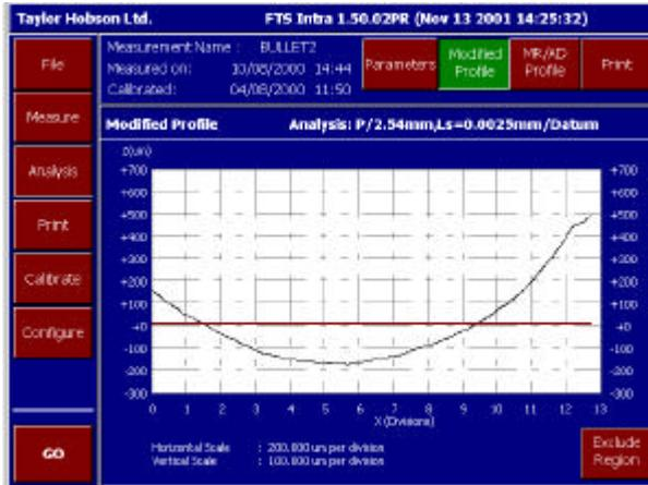
The Exclude Region option allows portions of the profile at either end of the profile to be excluded from any subsequent analysis, particularly a LS Arc analysis. Pressing the Exclude Region button enables the function and allows the Left Hand side Exclude Region to be changed using the < or > buttons.
