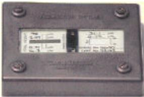
The Three Line and Ra Calibration Standard, for use with the Form Talysurf Intra instrument consists of a frame and base on which are mounted two glass plates.
