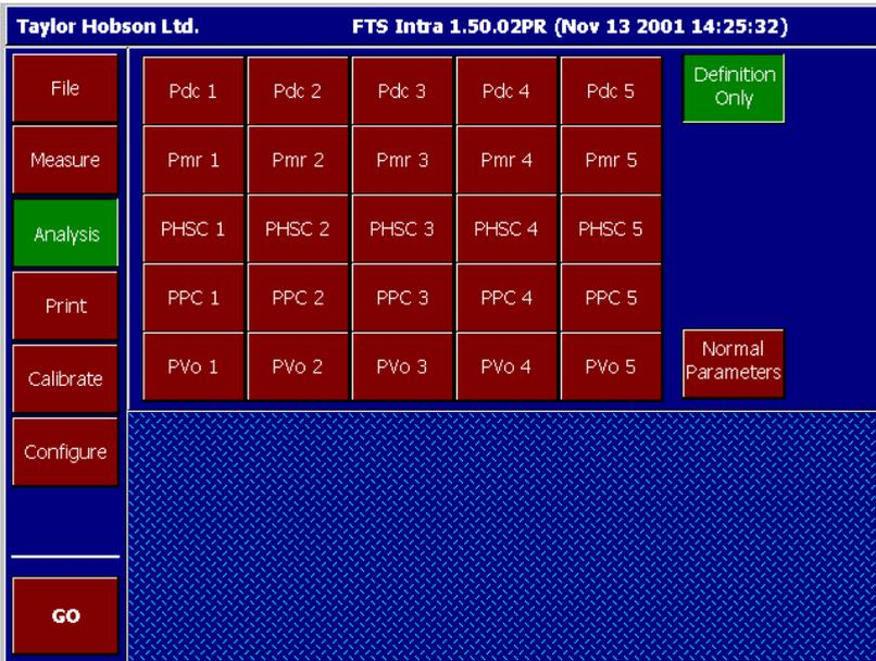
Parameter options are selected from the upper pane of this menu. The lower pane provides facilities for the display and input of user definitions. Only those selected will appear in the Results displays and be available for printing.
