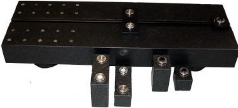
The base is a granite construction on anti-vibration mounts, and provides a firm support for the traverse unit and the various workpieces. The isolation from vibration provided by the base enables the system to be used up to maximum performance level close to normal engineering environments (this does not include high energy activity such as forging, planing, shearing, bending etc). One tee slot enables fixtures and base accessories to be secured to the surface.
