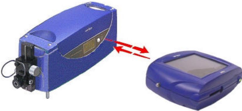
Designed to address a wide range of shop floor, production line and automated measurement applications, the instrument's accuracy and analysis capabilities also make it an invaluable addition to inspection and research laboratories (the instrument has a normal Gauge range of 1mm [0.039in] with a measurement resolution of 16 nanometres [0.63 $\mu$ in], but can have a reduced Gauge range of 200 $\mu$ m with a measurement resolution of 3.2nm).
