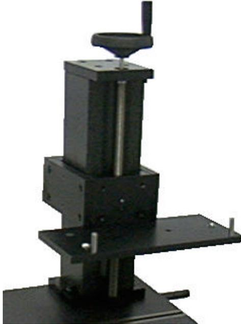
The column is used in conjunction with the Granite Base to provide a rigid stable mounting for the traverse unit. This enables the height of the traverse unit to be easily and precisely adjusted.
