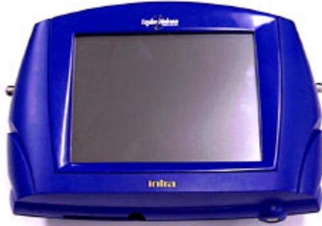
All instrument operation commands, analysis requirements and results displays are via a touch pad screen.
