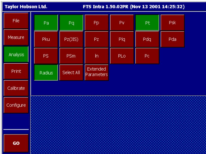
This menu consists of a button panel of normal parameter options, an **Extended Parameters** button (except on the Rk parameters menu) and a **Select All/ Select None** button. Parameters are selected for evaluation by pressing the relevant option buttons.
