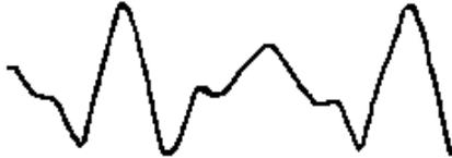
Note that not all components are in step with each other i.e. we need to know not only the amplitude of the component but also its phase in relation to the fundamental.
