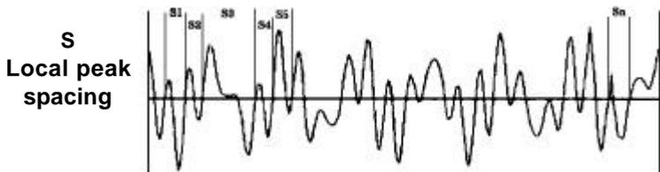
**RSm WSm PSm** - The mean spacing between profile peaks at the mean line, measured over the evaluation length. (A profile peak is the highest part of the profile between an upwards and downwards crossing of the mean line). There is a 10% z height discrimination and 1% sampling length spacing discrimination.
