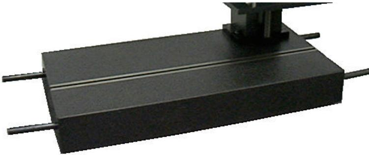
The base is of an epoxy granite construction on anti-vibration mounts, and provides a firm support for the column and workpieces. The isolation from vibration provided by the base enables the system to be used up to maximum performance level close to normal engineering environments (this does not include high energy activity such as forging, planing, shearing, bending etc). One tee slot enables fixtures and base accessories to be secured to the surface.
